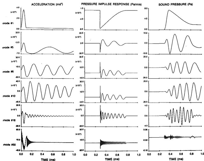
Fig. 2 The modal acceleration response, pressure impulse response, and corresponding sound pressure radiation for various modes of the plate.  $z = 0.10$  m,  $\xi = 0.025$ .
