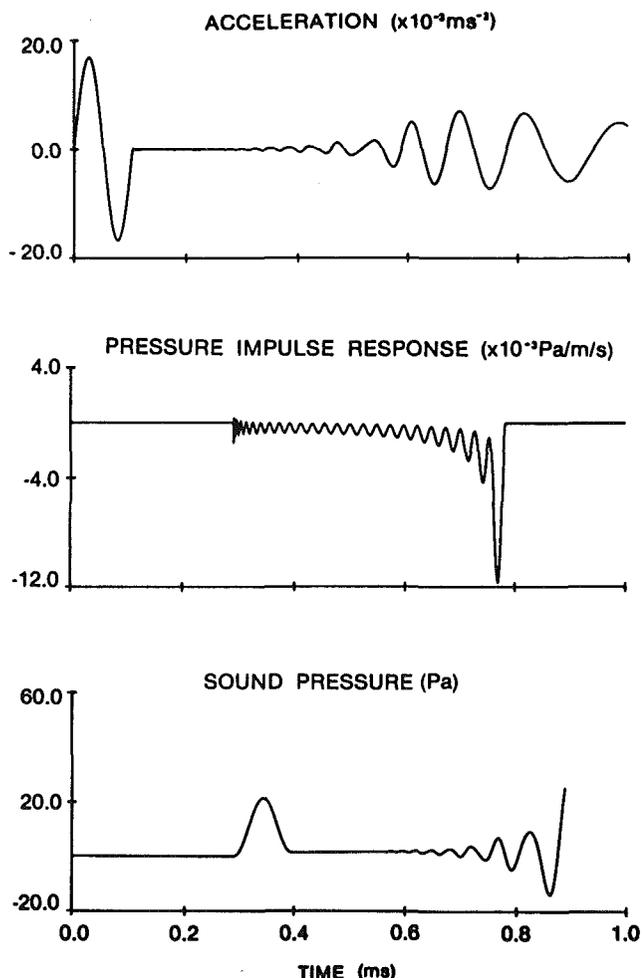
Fig. 3 The plate acceleration, pressure impulse response, and sound pressure obtained using the first 50 modes of the plate.  $z = 0.10$  m,  $\xi = 0.025$ .
