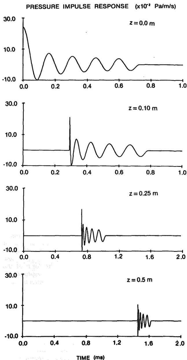
Fig. 4 The tenth modal pressure impulse response at various distances from the plate surface.  $\xi = 0.025$ .
